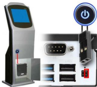
**External power button by separate remote line**
