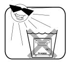
Do not block the air vents to this device or impede the airflow in any way.
