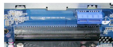
Two PCI-Express Slots: X16 and X1
